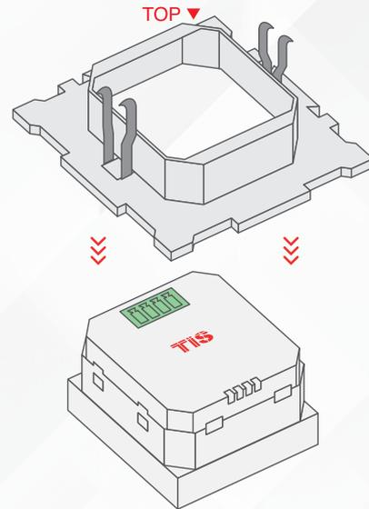
**3**» Connect the TIS-BUS Cable to the connector, and insert it into the Terre module.
