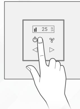
**3** Test your air conditioning by changing the fan speed from low to medium to high. Your relay should respond accordingly.
