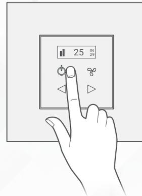
**3** Test your air conditioning by changing the mood, Heat/Cool, and fan speed from low to medium to high. HVAC module should respond accordingly.
