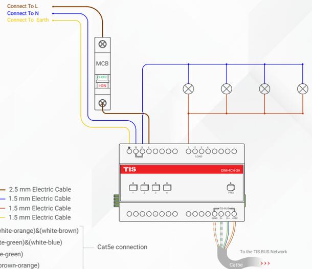
**6** Turn on the power source, and then test the loads by short pressing on local override buttons 1-4 on the device.
