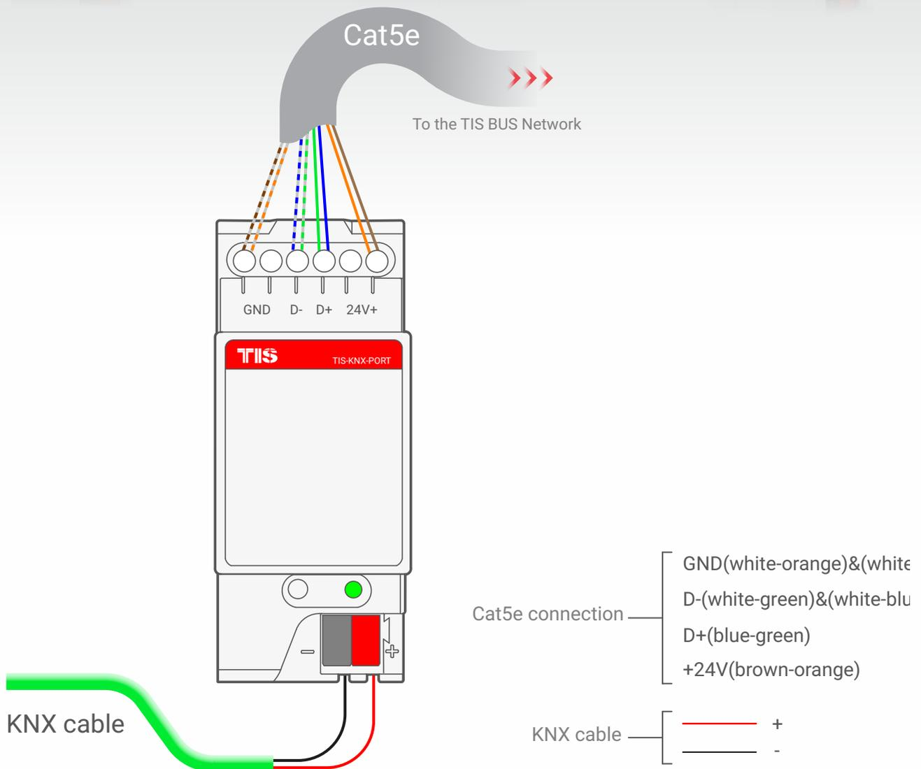
▲ Figure 1: TIS BUS-KNX Converter Configuration Diagram
