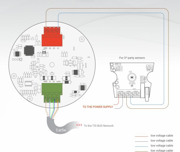
Figure 1: 3<sup>rd</sup> Party Sensor Connection Diagram
