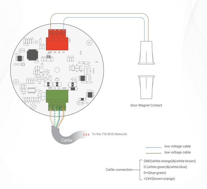
**Figure 3: Magnetic Door Contact Connection Diagram**
