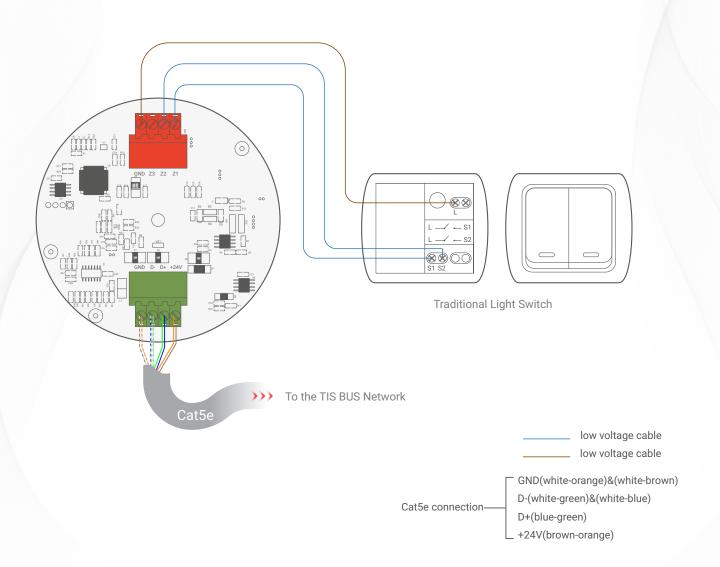
Figure 2: Traditional Light Switch Connection Diagram
